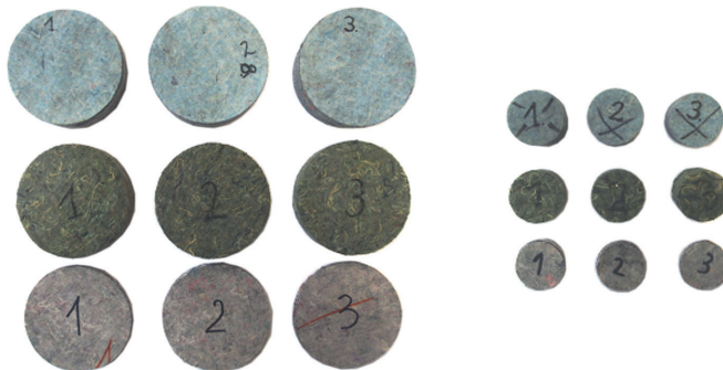
Fig. 1. Samples: \varnothing 100\text{mm} - left view, \varnothing 30\text{mm} - right view (from up: blue poroso, green poroso and thin poroso)
