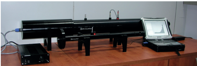
Fig. 2 Apparatus for determining the sound absorption coefficient – impedance tube
