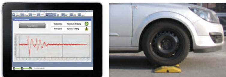
Fig 4. Investigating of the condition of shock absorbers using a body acceleration sensor. Vibration recording with a PTI tester [8]
