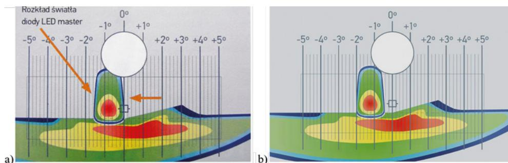
Fig. 2. Control of light distribution of the LED master in LED reflector Matrix. a) location of the field illuminated by the master diode – correct, b) incorrect [11]
