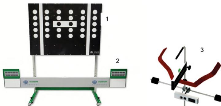
Fig. 3. The stand for tests of the setting and calibration of cameras for the control of the driving path. 1 - calibration board, 2 - screens for setting the board relative to the vehicle body, 3 - holder for fixing the laser pointer to the tire of the vehicle wheel [12]
