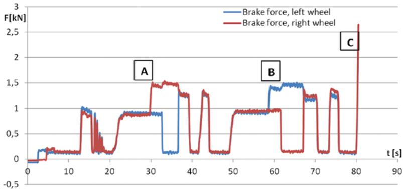
Fig. 5. Example of valve and ABS pump system control of the rear axle of a passenger car.  $F$  – braking force,  $t$  – measurement time. Description in the text.
