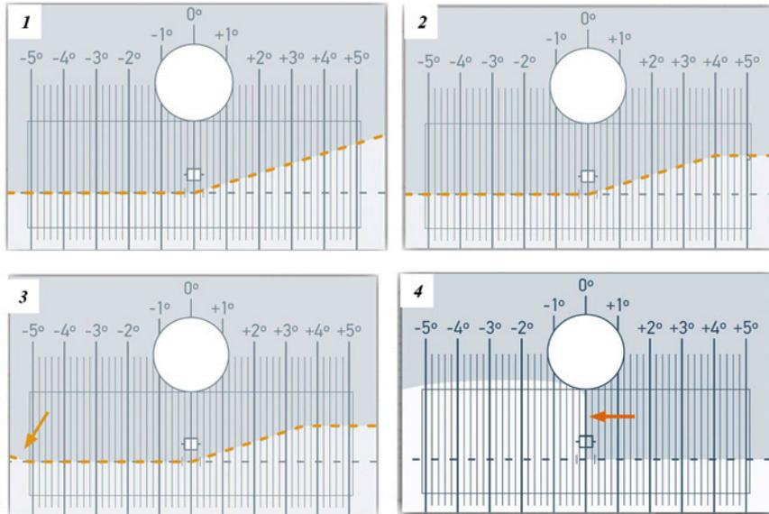
Fig. 1. Differences between the light and shadow boundary of the low beam: 1 – headlamps with halogen bulbs, angle of elevation of the light and shadow boundary 15°, 2 – reflector with discharge lamps, angle 12° (up to 75°) and limitation of heights, 3 – headlights with LED diodes, angle of elevation 12° (up to 75°), limitation of elevation of the shadow border on the left, 4 – limit of light and shadow of headlights in the car with the assistant of high beam [10, 11]
