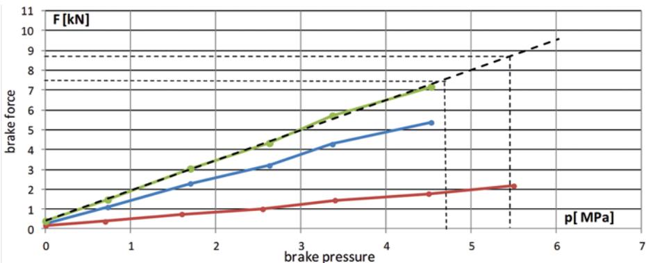
Fig. 6. Results of measurement of braking forces as a function of pressure in the passenger car's braking system. — front brakes, — rear brakes, — sum of forces, - - - regression function and values of forces and pressure necessary to achieve the required braking performance of 50% and 58% for the tested vehicle with a mass of dmc 1500 kg
