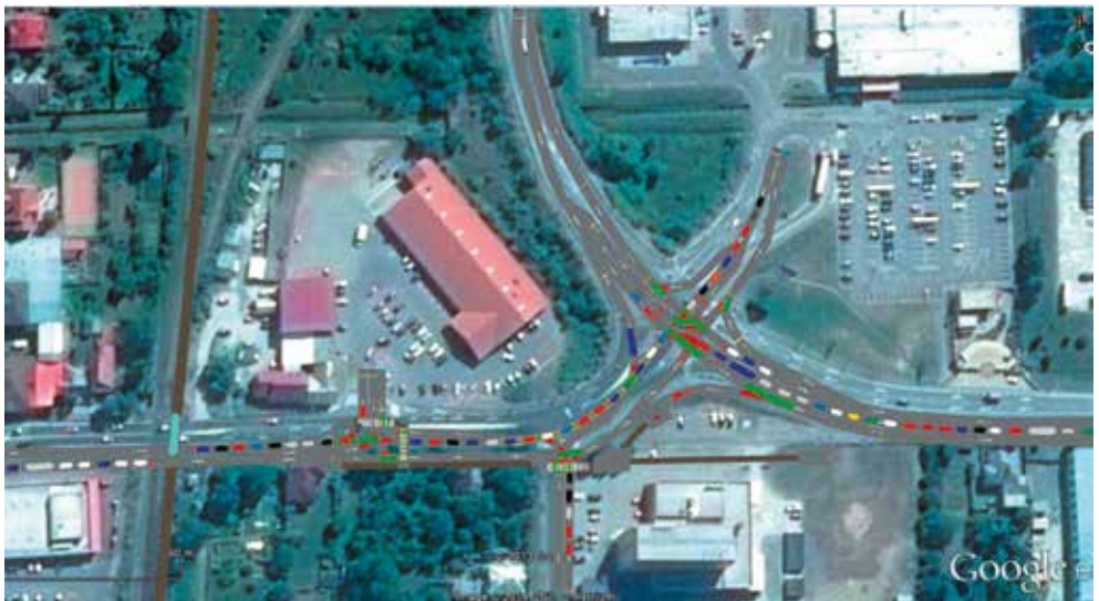
Fig. 3 Illustration of traffic situation in the town Vranov nad Toplou obtained from simulation of the traffic status in case of the closed grade crossing
