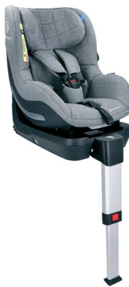
**Fig. 4. Child seat "I" mounted on the ISOFIX base, facing the direction of travel [6]**
