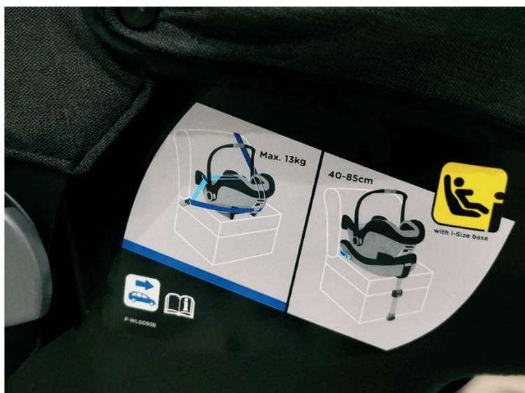
**Fig. 2. Marking of the methods of mounting the child seat of the youngest group in a passenger vehicle**
