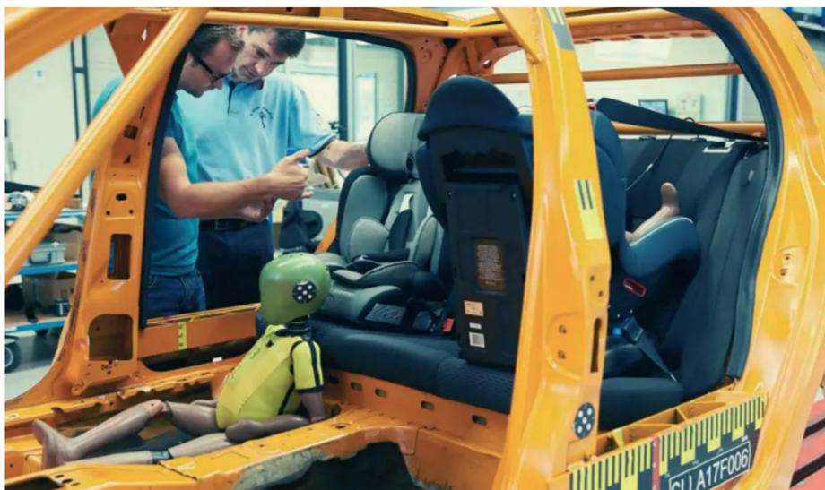
Fig. 5. Crash test frame of ADAC vehicle seats [8]
