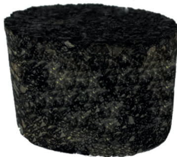
Fig. 2. The sample prepared for the application of the braking trace
